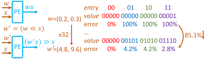
Fig. 10. Pre-scaled weight scaling scheme.
